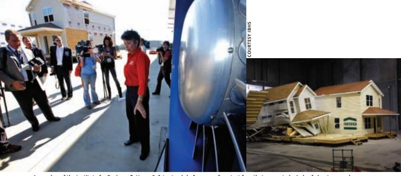
A member of the Institute for Business & Home Safety stands before one of 105 test fans that generated winds of about 100 mph. Above right: While the house without fortification collapsed after high winds, the fortified home remained intact.
