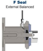
Externally balanced D or DG Seal with water cascade for use when normal D seal applications include product temperatures that reach 212°F or when the fluid is sticky or tacky.
