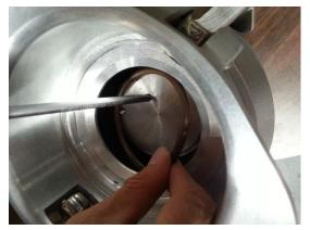
Note! After the O-Ring (8) is removed, the poppet stop (12) will hold the poppet (3) in the coupler body. If the poppet (3) is worn or damaged, remove the coupler from the hose or the mating part.
