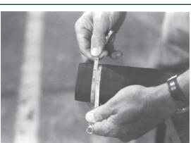
Accurately measure the hose O.D. with a diameter tape. Select the correct Holedall  $^{\text{TM}}$  Petroleum Ferrule from the DPL based upon the Hose O.D. just measured.
