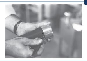
Make sure the hose end is cut square. Slide the ferrule over the hose until the turned over end of the ferrule contacts the end of the hose. Place a mark on the hose at the junction of the ferrule and hose. Move the ferrule away from the hose end  $\frac{1}{6}$ " and place another mark at the junction of the hose and ferrule. This will insure that the proper rubber displacement or pocket is maintained during the expansion process.
