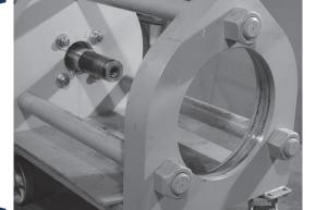
Install IX Master Plate onto outside of ram die bed. Position the bolt holes at the 3 o'clock and 9 o'clock positions. Secure with straps and bolts by positioning the straps on the inside of the die bed. Tighten the nuts on the bolts.
