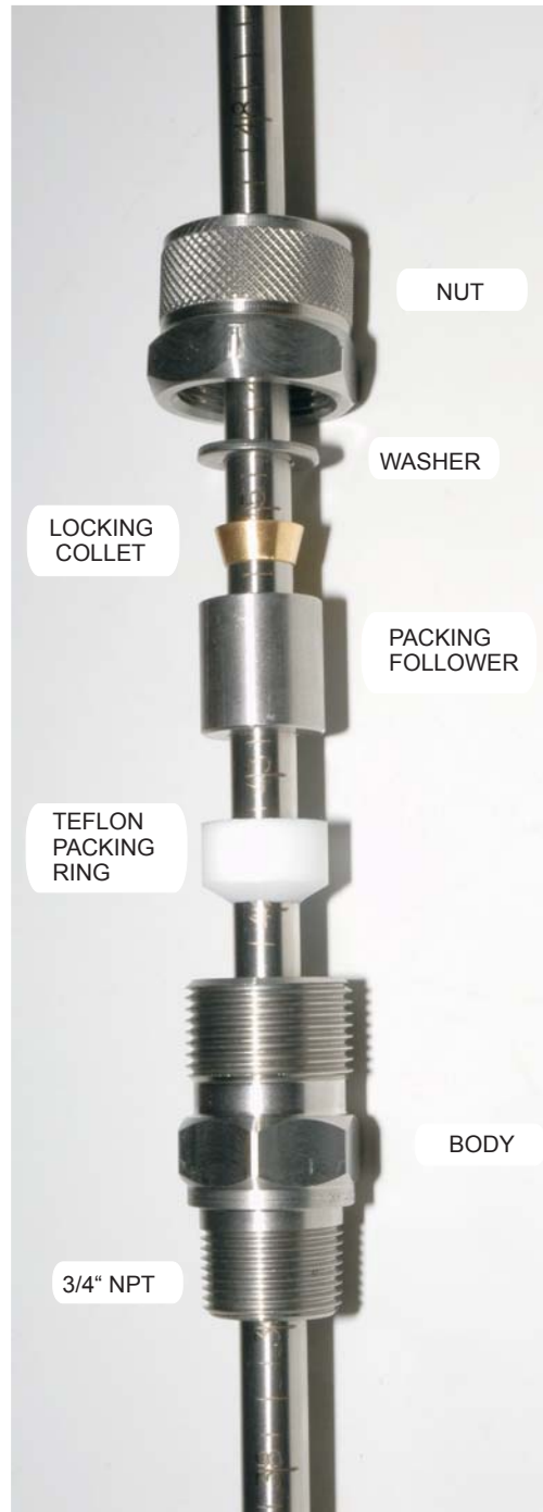
EXPLODED VIEW, 3/4" 300 LB SLIDING FITTING
