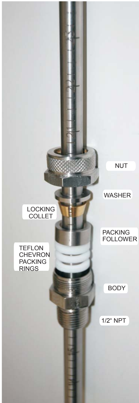
EXPLODED VIEW, 1/2" 150 LB SLIDING FITTING
