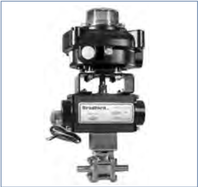
Bradford™ automated 1/2" encapsulated 2-way ball valve buttweld ends spring return actuator and NEMA 7 (explosion proof) SPDT limit switch with two proximity switches and NEMA 7 NAMUR mount 24VDC voltage solenoid valve pictured. BV2CV-050BB-FPC.
