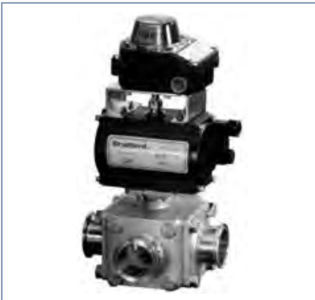
Bradford™ automated 1½" 3-way 'L'-port encapsulated hygienic ball valve with double acting actuator and NEMA 4 limit switch with two SPDT mechanical switches and NEMA 4 115 VAC solenoid pictured. BV3SVLF150CBXC .
