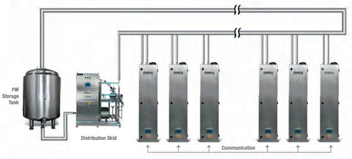
When multiple POUs are installed in series on loop, the simultaneous operation of POUs is controlled to ensure the minimum required loop velocity as per Pharmaceutical guidelines. This is achieved by the POU to POU communication feature in which all POUs communicate with each other using Ethernet protocol. The user can limit the maximum number of POUs in operation to ensure the loop velocity is maintained
