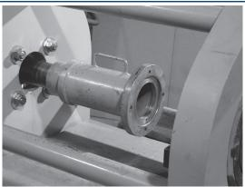
Install the Cam & Groove pusher necessary to do the size and style of coupling to be swaged into the Main Pusher (M011-065). Additional pushers may be required. Reference the chart at the end of this section for proper pusher selection.
