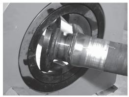
Loosen the bolt(s) on the tie down bar(s) and move the tie down bar(s) so that they clear one die bed spacer. Tighten any bolt just loosened. Remove the die bed spacer one half at a time. Repeat this process for each die bed spacer to be removed. Remove only enough die bed spacers to allow the flange to pass through.
