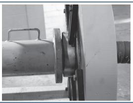
Depress and hold the button on the remote until the wing nut (or spacer) contacts the die face. Release the button. Return the directional control lever to the "NEUTRAL" position.
