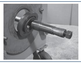
Slide the stem over the Pull Rod and into the recess of the Thrust Plate with the connection side of the stem facing the ram. For male stems, insert the hex into the recess of the Thrust Plate. For female stems, insert the first hex into the Thrust Plate so that the second hex will fit into the recess of the Thrust Plate.
