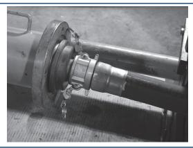
Move the directional control lever to the "FORWARD" position. Depress the button on the remote and advance the cylinder until the end of the ferrule is near the die opening. Using a wooden board or metal pipe, lift the ferrule up. Jog the cylinder by quickly depressing and releasing the button on the remote. This will allow the ferrule to enter the die slowly without contacting the die face. Continue jogging the cylinder until the ferrule has entered the die approximately one half inch.
