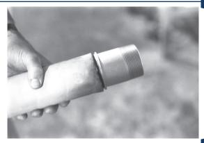
Lubricate the I.D. of the hose and the O.D. of the stem with Dixon Coupling Lubricant or equivalent. Insert the stem all the way into the hose until the ring on the stem comes in contact with the end of the hose.
