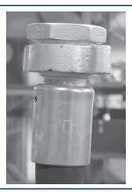
Lubricate the I.D. of the hose and the O.D. of the stem (as well as possible) with Dixon Coupling Lubricant or equivalent. Insert the stem all the way until the mark on the hose (from Step 4a) is at the end of the ferrule.
