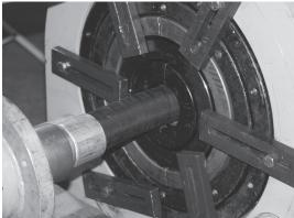
Loosen and move any tie down bars that may come in contact with the coupler head. Depress and hold the button on the remote until the spacer rings are even with or about to contact the die face. Release the button on the remote. Return the directional control lever to the "NEUTRAL" position.
