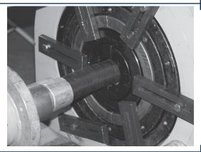
While holding the die in place with one hand, place one of the tie down bars over the die so that it does not come out of the die holder unexpectedly. Secure the tie down bar by tightening the bolt.
