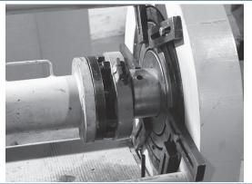
Move the directional control lever to the "Forward" position and depress the button on the remote. Advance the cylinder forward until the end of the ferrule is near the die opening. Using a wooden board or metal pipe, lift the ferrule up. Jog the cylinder by depressing and releasing the button on the remote. This will allow the ferrule to enter the die slowly. After the ferrule has entered the die, stop advancing the cylinder.
