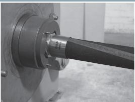
**Note:** If the gauge reads 10,000 PSI before internal expansion is complete, stop. Contact Dixon for further assistance. During internal expansion never stand directly in front of the ram. Visually inspect the coupling.
