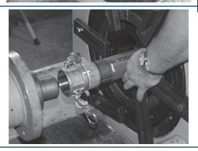
Move the directional control lever to the "REVERSE" position. Depress and hold the button on the remote retracting the cylinder until there is sufficient room for the stem and ferrule to clear the die bed.
