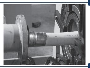
Move the directional control lever to the "REVERSE" position and depress the button on the remote. Retract the cylinder far enough (approximately 1") to allow a tie down bar be placed so that the die does not come out of the die holder. Secure the tie down bar by tightening the bolt. Continue retracting the cylinder until there is sufficient room for the stem and ferrule to clear the die bed.
