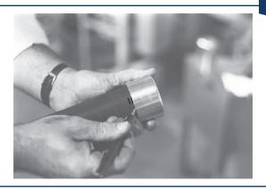
Make sure the hose end is cut square. Slide the ferrule over the hose until the turned over end of the ferrule contacts the end of the hose. Place a mark on the hose at the junction of the ferrule and hose. Move the ferrule away from the hose end \(^1/8\)" and place another mark at the junction of the hose and ferrule. This will insure that the proper rubber displacement or pocket is maintained during the expansion process.
