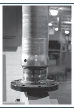
Wipe excess lubricant from hose and ferrule. Bring hose with stem and ferrule back through die bed.
