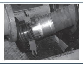
Position a rubber sheet or pad under the die bed. <u>Slowly</u> slide the hose towards the pusher. When the die clears the die holder, one or both halves may fall to the floor. If one half remains on the ferrule, tap it with a mallet until it releases. If both halves remain on the ferrule, it may require the halves be pried apart at the seam.
