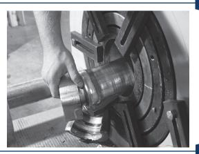
Install the required die holders ensuring that the seams between the die holder halves do not line up. The die holders are designed to fit one inside the other.
