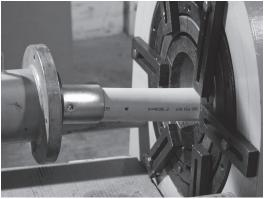
Lifting up the hose, insert one die half under the hose. Lower the hose so that it rests on the die. Insert the other die half. Make sure that the seams of the die do not line up with the seams on the die holders.
