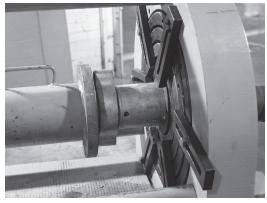
Align the wing nut (or spud) with the pusher ensuring they are flush with each other. Jog the cylinder forward until pressure begins to register on the gauge. Leave the directional control lever in the "FORWARD" position. Check the alignment between pusher and wing nut (or spud). If any adjustment is necessary, do it now.
