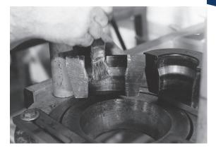
Lubricate the I.D. of both die halves with  $Crisco^{\otimes}$  (recommended) or high viscosity oil or heavy duty grease.
