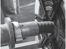
Bring the hose with the stem and ferrule through the die bed. Position the wing nut (or spud) as close to the pusher as possible. Make sure that there is sufficient room between the die holders and the end of the ferrule to comfortably insert the die halves into the die holders.
