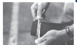
Accurately measure the hose O.D. with a diameter tape. Select the correct Holedall  $^{\text{TM}}$  Petroleum Ferrule from the DPL based upon the Hose O.D. just measured.
