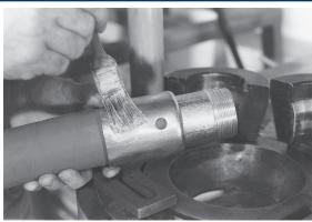
Lubricate the outside of the ferrule with  ${\sf Crisco}^{\otimes}$  (recommended) or high viscosity oil or heavy duty grease.
