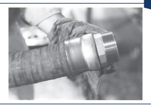
Lubricate the O.D. of the stem and the I.D. of the hose with Dixon lubricant or equivalent. Insert the end of the fitting into the hose. Assemble the ferrule onto stem by sliding turned over portion of ferrule past notched section of stem collar. Rotate ferrule  $90^{\circ}$  (¼ turn). With ferrule and stem engaged, continue installing stem until ferrule reaches the second mark on the hose.
