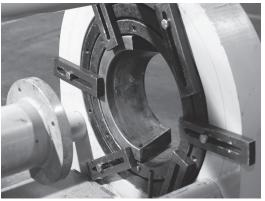
Secure the die holders with tie down bars to prevent the die holders from slipping out of the die bed unexpectedly.
