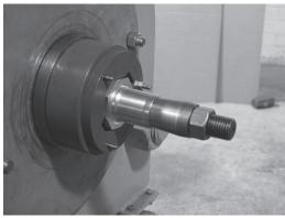
Screw or slide the IX plug, small end first, onto the Pull Rod and into the shank of the stem. For 2" and above screw the retaining nut on until it contacts the plug. Move the stem slightly to allow for slack and hand tighten the plug or nut until it is snug.
