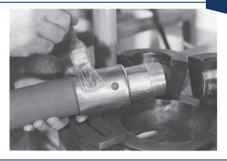
Lubricate the outside of the ferrule with Crisco® (recommended) or high viscosity oil or heavy duty grease.
