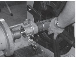
Move the directional control lever to the "REVERSE" position. Depress and hold the button on the remote retracting the cylinder until there is sufficient room for the stem and ferrule to clear the die bed.
