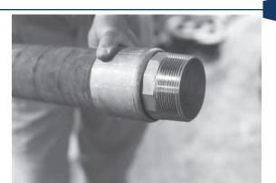
Lubricate the O.D. of the stem and the I.D. of the hose with Dixon lubricant or equivalent. Insert the end of the fitting into the hose. Assemble the ferrule onto stem by sliding turned over portion of ferrule past notched section of stem collar. Rotate ferrule 90° (¼ turn). With ferrule and stem engaged, continue installing stem until ferrule reaches the second mark on the hose.
