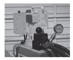
On-Off-Remote switch, 0 - 10,000 PSI pressure gage and hand held remote.
