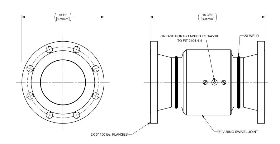
\*SWIVEL WILL BE SHIPPED W/ 2X 2404-4-4 INSTALLED AND CAPPED ON JIC END.
