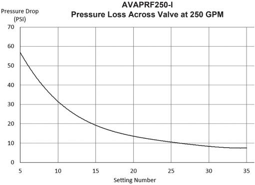
Readings based on flow held to 250 GPM and outlet pressures of **100**, **110**, **120**, and **150 PSI**. Example: Inlet Pressure **120 PSI**, Discharge Pressure **100 PSI** - the Set Number should be 15
