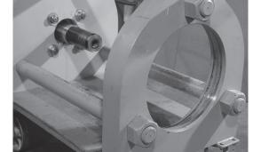
Install IX Master Plate onto outside of ram die bed. Position the bolt holes at the 3 o'clock and 9 o'clock positions. Secure with straps and bolts by positioning the straps on the inside of the die bed. Tighten the nuts on the bolts.
