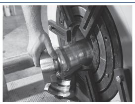
Reposition the tie down bars on the die face so that the wing nut (or spacer) will clear.
