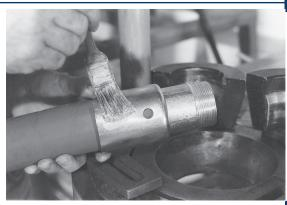
Lubricate the outside of the ferrule with  ${\sf Crisco}^{\$}$  (recommended) or high viscosity oil or heavy duty grease.
