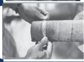
Slide the ferrule all the way onto the hose. Place a mark on the hose at the end of the ferrule. Move the ferrule ½" from the mark just made towards the end of the hose. Place a second mark on the hose at the end of the ferrule.
