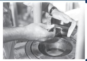
Lubricate the I.D. of both die halves with  $\textsc{Crisco}^{\textsc{@}}$  (recommended) or high viscosity oil or heavy duty grease.
