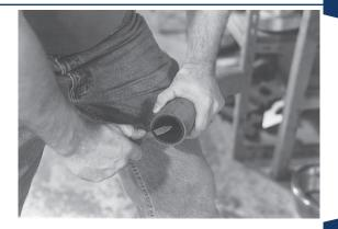
Assuring that the hose end is cut square, chamfer the I.D. of the hose  $\frac{1}{6}$ " at a 45° angle. This will aid in stem insertion. If the hose is to be static grounded, follow hose manufacturers procedure for proper static grounding.
