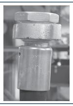
Lubricate the I.D. of the hose and the O.D. of the stem (as well as possible) with Dixon Coupling Lubricant or equivalent. Insert the stem all the way until the mark on the hose (from Step 4a) is at the end of the ferrule.
