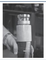
Place a mark on the outside of the ferrule that corresponds with the center of one of the turned over sections of the ferrule. This mark will act a guide for correct engagement with the stem collar.
